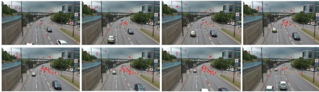
Fig. 1 Centroids on holes in a sequence of video frames. Each + (red plus sign) identifies the centroid of a hole. The locations of the holes in these video frames vary from moment due varying atmospheric conditions. (Color figure online)
